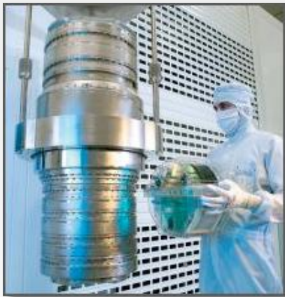
Lenses for Computer Chip Manufacturing
