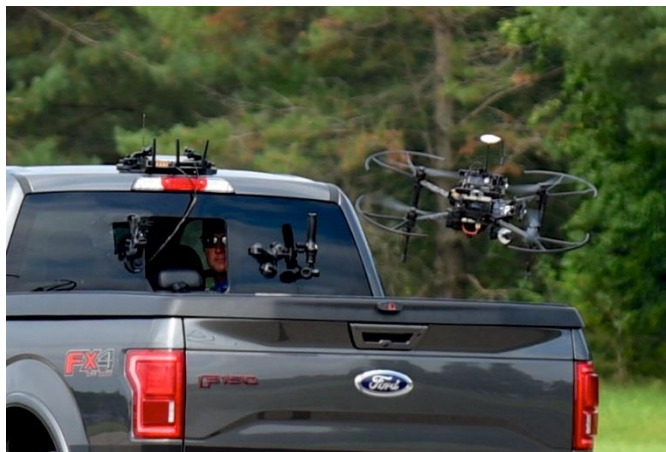
A DJI UAS autonomously launches from the bed of a moving Ford pickup truck on its way to a simulated disaster site during the 2016 Developer Challenge at Griffiss International Airport in Rome. Credit: Eric Miller, NUAIR
