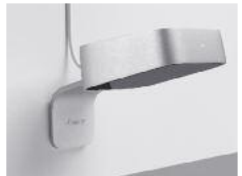
Density uses state-of-the-art depth data, computer vision, and deep learning to measure the real-time occupancy of spaces. Photo credit: Density
